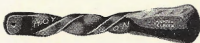
Sample bar of NUMBER ELEVEN Metal, bent, twisted and hammered cold, demonstrating its exceptional toughness.
